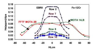
Fig. 3. Calculated He/dpa ratios for Fe–12Cr irradiated in EBR-II and FFTF. The earlier EBR-II experiment was conducted in-core in row 2 at  $\sim$ 0.18 appm He/dpa while the current FFTF experiment was conducted both in and out-of-core, with He/dpa ratios falling from 0.08 to 0.02 appm/dpa.
