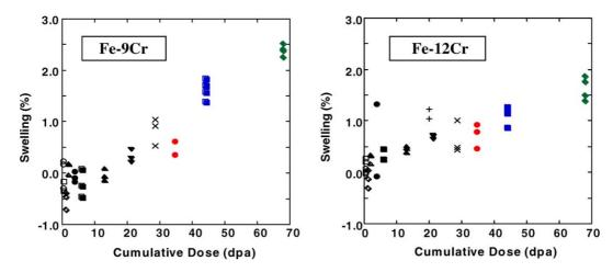
Fig. 2. Swelling of two simple model bcc Fe–Cr alloys in FFTF-MOTA at  $\sim$ 400 °C, as observed in the current experiment, showing some early densification but no apparent dependence of swelling on dpa rate.
