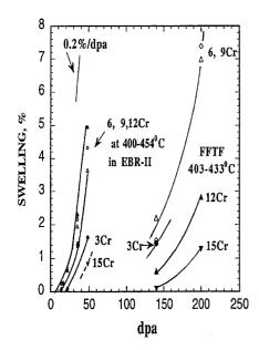
Fig. 1. Comparison of swelling of Fe–Cr binary alloys at  $\sim$ 400 °C in in-core regions of EBR-II and FFTF, as observed by Garner et al. [1].
